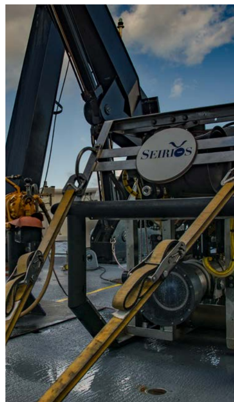
The forward-facing high-definition camera is the most commonly seen view from ROV Seirios . Image courtesy of NOAA OER, Deep-Sea Symphony: Exploring the Musicians Seamounts. http://oceanexplorer.noaa.gov/okeanos/explorations/ex1708/logs/sept26/media/camera.html
