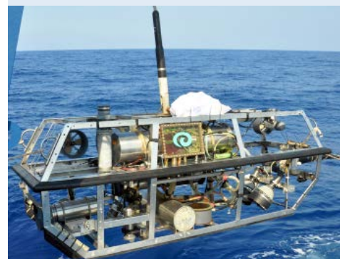
Argus (right) acts as a stabilizing platform for Hercules , following the ROV into the water. Image courtesy of The Ocean Exploration Trust.
