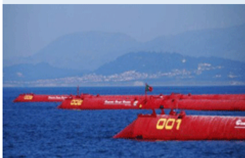
An attenuator device
