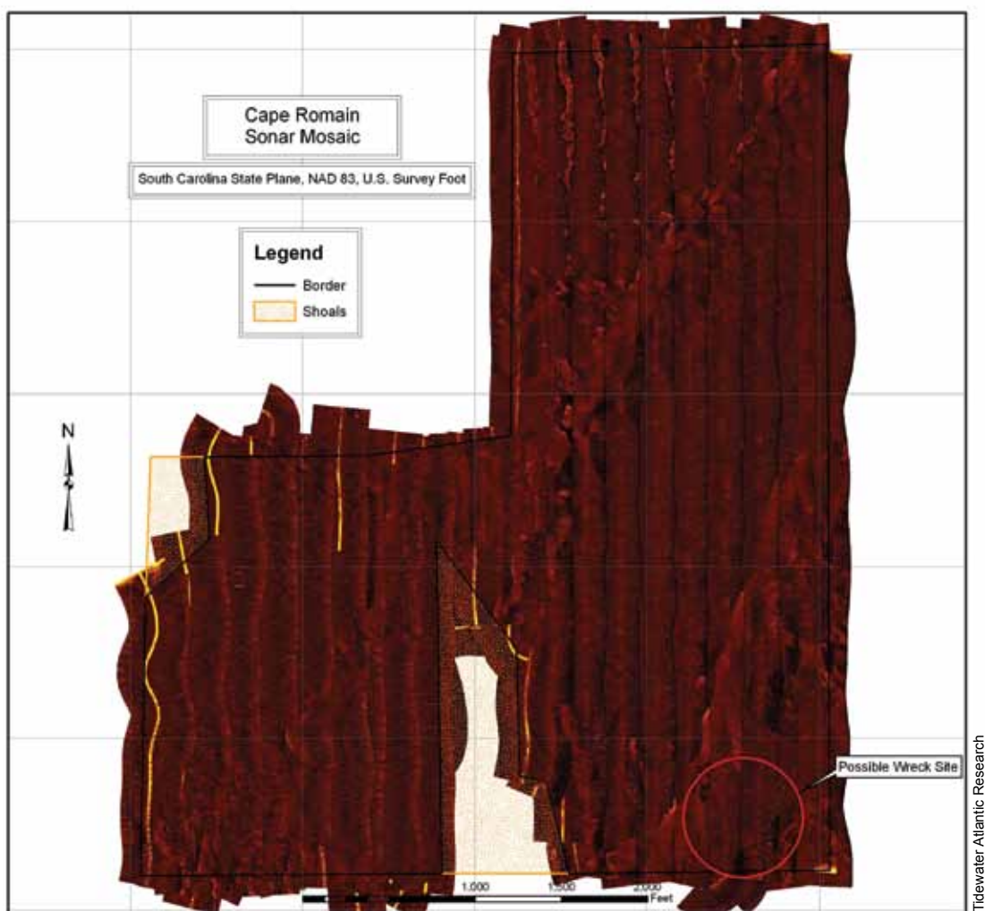
Figure 18. Sonar Coverage Mosaic of survey area (Coordinates redacted).
