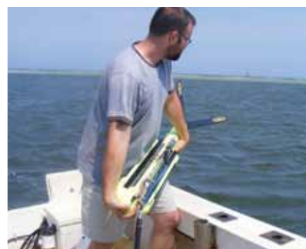
Figure 16. Launching the EG&G GEOMETRICS G-881 cesium vapor magnetometer.
