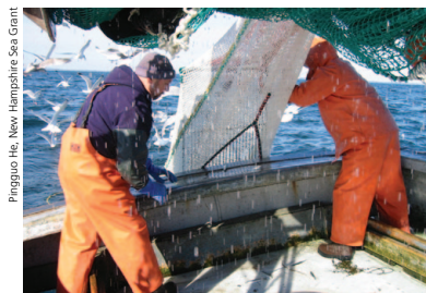
▲ Dave Goethal, left, a fisherman in Hampton, N.H., and deck hand Paul Kuncho hauling back one of a new topless shrimp trawl designed to reduce finfish bycatch in the pink shrimp fishery in the Gulf of Maine. New Hampshire Sea Grant collaborated with Goethal on the design, and secured funds from NOAA’s National Marine Fisheries Service to make several topless trawls for demonstration purposes. The trawl has reduced Gulf of Maine herring by-catch by 90% without loss of shrimp.
