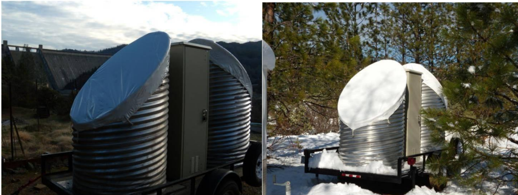
Figure 1. Snow level radar installations at Lake Shasta (left) and Colfax (right).
