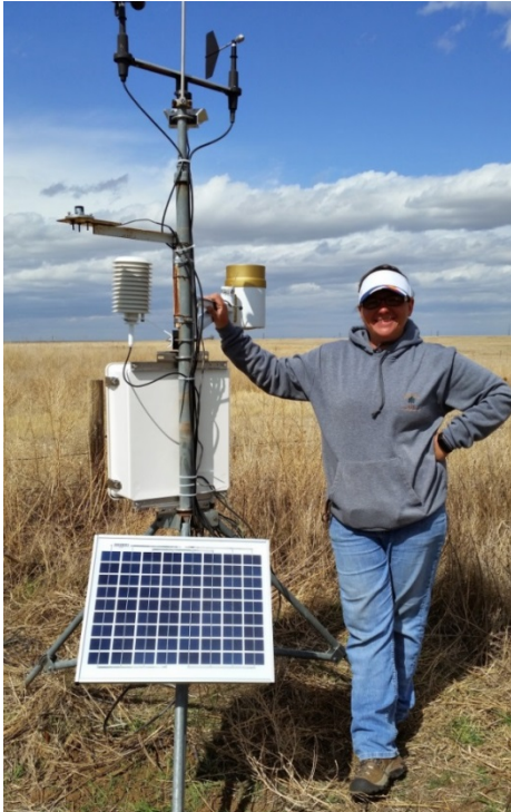
Wendy Ryan, Colorado Assistant State Climatologist, shows off a new CoAgMet station in eastern Colorado. Wendy has worked hard for several years to improve the quality of CoAgMet data.
