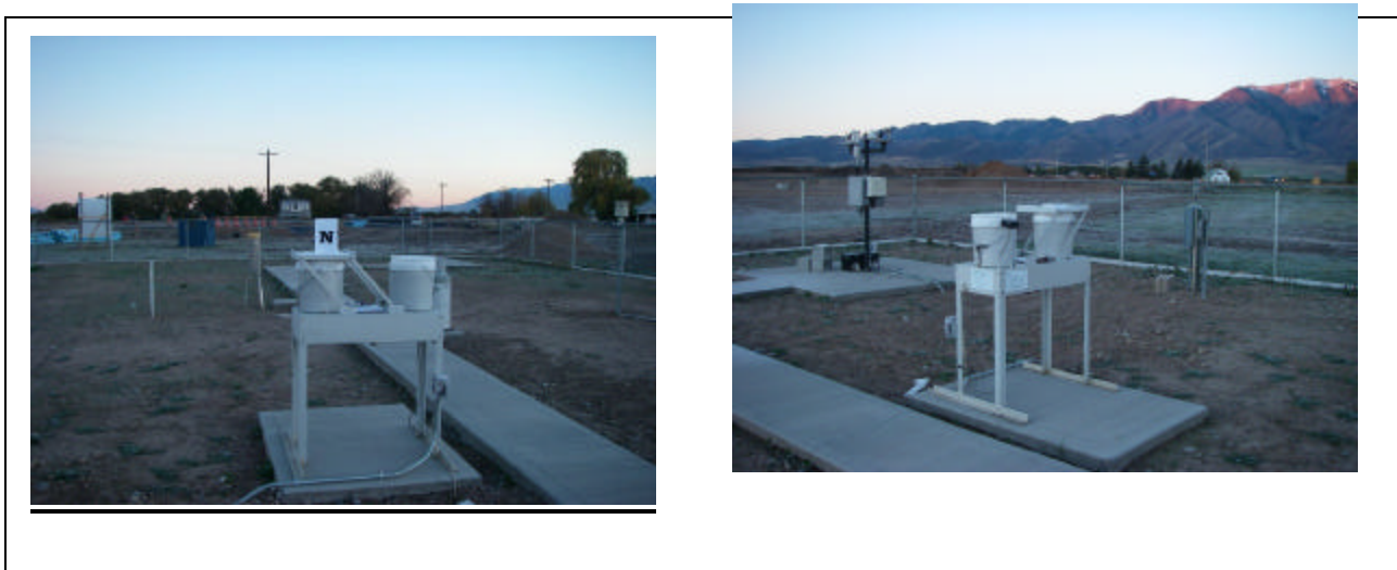
The new site for the COOP, NADP, and UVB stations at 5SW in Logan. Left-hand picture (looking North) shows NADP, COOP (MMTS, rain-gauge), while right-hand picture (looking Southwest) shows the UVB instrumentation.
