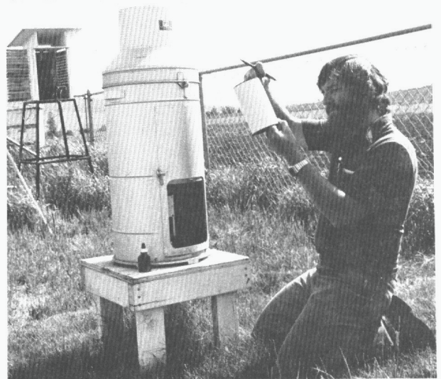
Hydrologic technician removing a raingage chart at a research site. The automated station is in the background.
