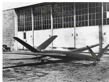
Figure 2. Michigan State Maritime Archaeologist Wayne Lusardi investigates the only aircraft found during the survey, a military tow target from the 1950s. Courtesy of John Bright, Thunder Bay National Marine Sanctuary . INSET. Schweizer Aircraft Corporation of Elmira, New York, manufactured 400 tow targets for the US Navy in the 1950s. How this particular target ended up in Lake Huron is unknown. Courtesy of Paul Schweizer, Schweizer Aircraft Corporation
