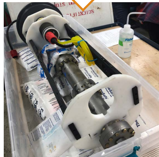
Figure 2. The pressure-retaining seawater sampler outside of its housing. Image credit: Doug Bartlett, Scripps Institution of Oceanography
