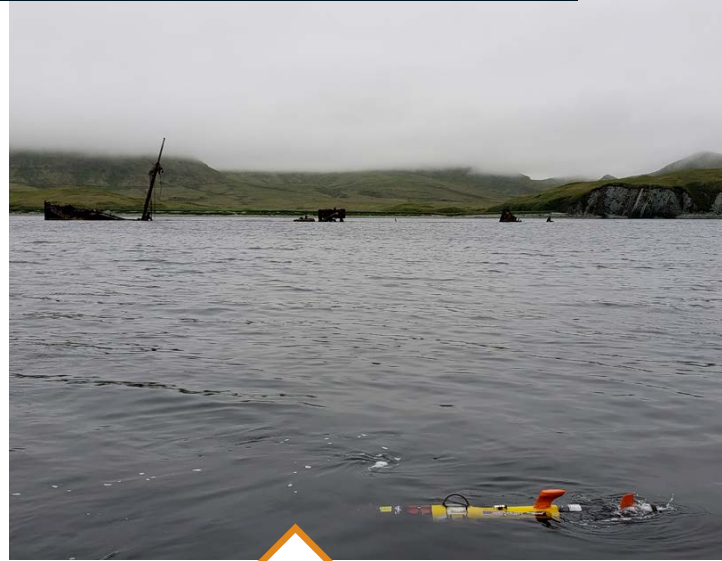
Figure 2. One of four REMUS 100 UUVs utilized during the Kiska survey to image the seafloor to detect potential archaeological sites. Courtesy of Kiska: Alaska's Underwater Battlefield expedition, Scripps Institution of Oceanography
