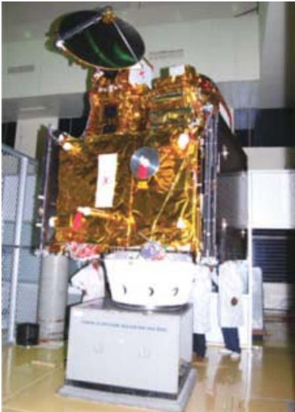
Oceansat-2 undergoing dynamic balancing test
