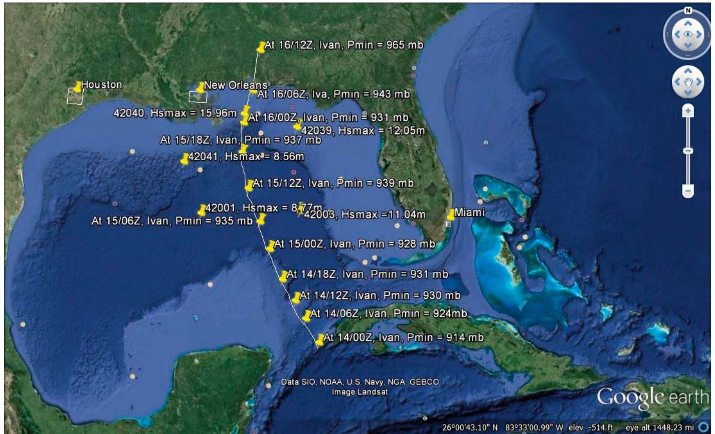
Figure 2. Ivan’s track over the Gulf of Mexico and its maximum significant wave heights measured at 5 NDBC buoys. For the entire track history (see www.nhc.noaa.gov ).
