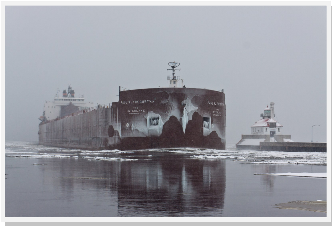
This is a photo of the Paul R. Tregurtha (also known as the “Queen of the Lakes”) as she is the longest ore freighter trading across the Great Lakes with a length of 1013 ft. She was built in 1981, and of significance is she is our newest bulk carrier on the American Fleet. Our ships on the Great Lakes for the American side do not trade in salt water, so the longevity of these ships is quite long. We still have ships that are built around the turn of the 20 th century and many around 1950 circa. This photo looks to be in late December with the start of the ice season on the Great Lakes.
