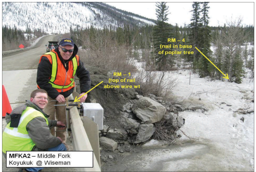
Forecaster Ray Little (left) and Observation Program Leader Brad Sipperly perform routine maintenance on a wire weight gage located on the Middle Fork of the Koyukuk River. Both Ray and Brad work in the Fairbanks WFO.
