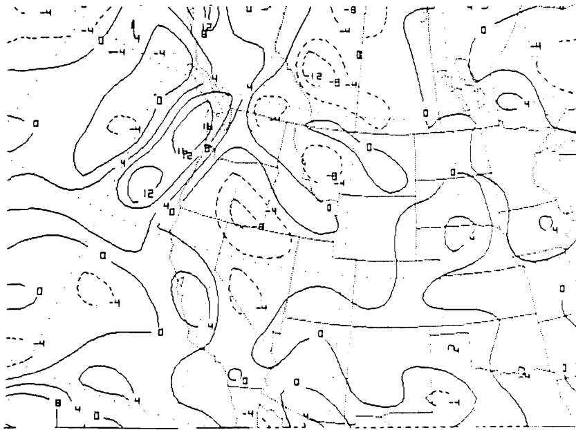
Figure 3. NGM 06 hour forecast of layer-averaged Q-vector divergence (solid) and convergence (dashed) valid at 1800 UTC 27 May 1994. Divergence of Q is solid and convergence of Q is dashed. Layer-average is centered at 500 mb and extends from 700 to 400 mb. Contours at 4 \times 10^{-15} \text{ mb}^{-1} \text{ s}^{-3} . (Static stability is not involved in calculation.)
