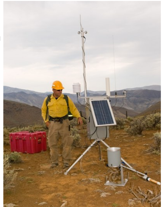
Electronics Technician next to a portable RAWS.
