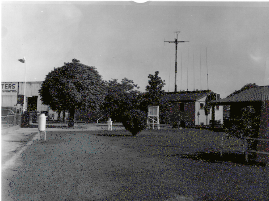
Figure3 - Weather instruments at the National Weather Service Office in Bakersfield. Two rain gauges and a cotton region shelter can be in this photograph taken in July 1950 (Photo courtesy NCDC).
