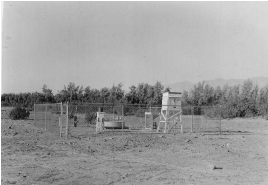
View of the weather station after moving to the Visitor Center at Furnace Creek. The instrument shelter, evaporation pan and rain gauge can all be seen in this photograph. Photo taken in August 1961 after a four and a half foot tall chain link fence was installed around the weather station. Photo Credit: NWS Las Vegas archives.
