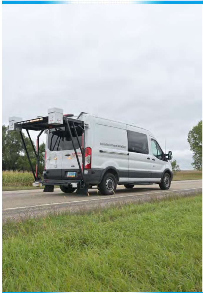
Automated Road and Pavement Condition Surveys vehicle that uses cameras and lasers to record the condition of the pavement
