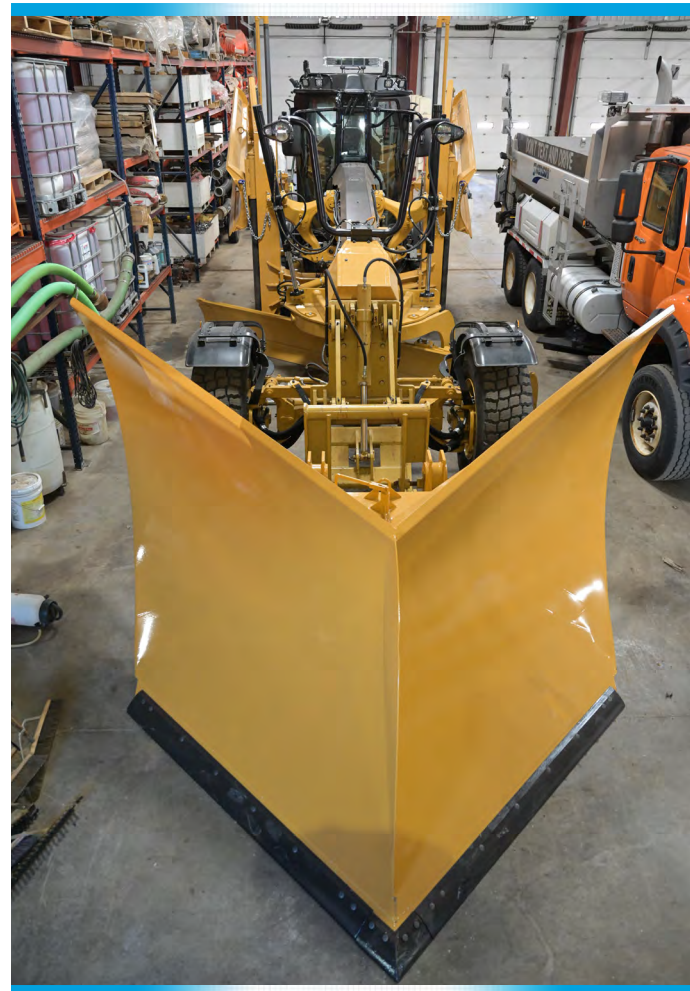
Maintenance's new V Plow vehicle that will be used on clearing large compacted snow drifts especially under underpasses
