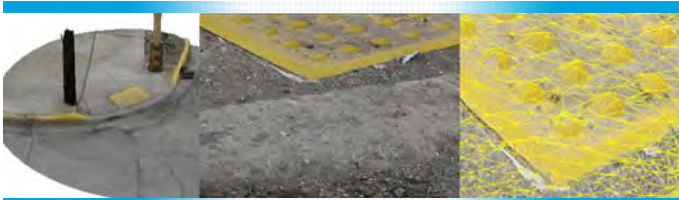
Left: 3D photograph of curb ramp. Middle: Zoomed in image of truncated dome and curb. Right: Final product Reality Mesh
