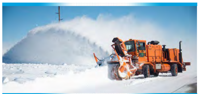
Clearing snow with a rotor plow after a big storm
