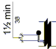
Figure 505.6 Horizontal Projections Below Gripping Surface
