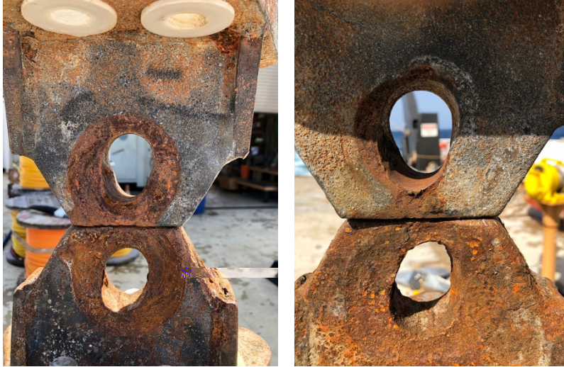
Figure 3 Wear on mooring bridle yokes.
