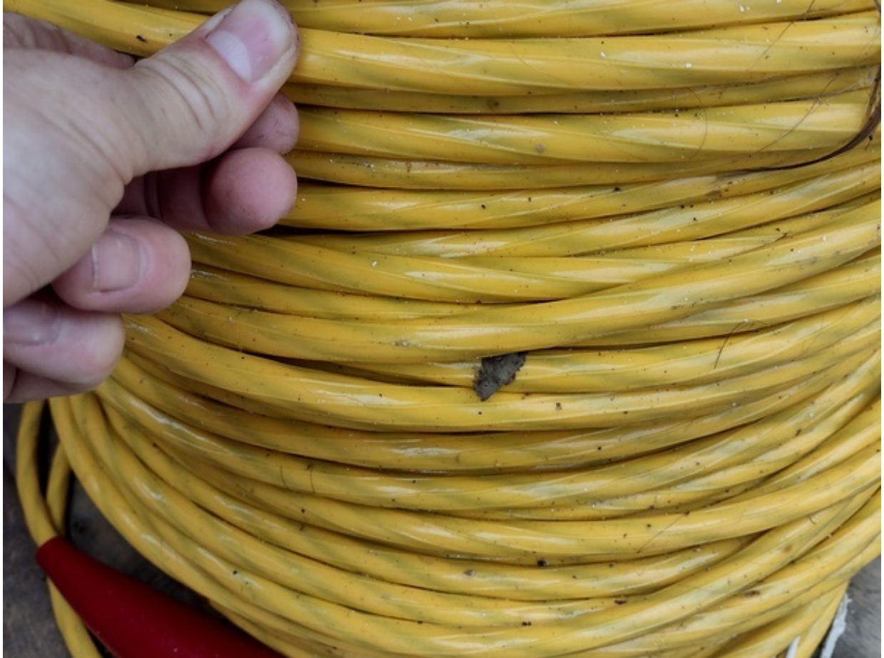
Figure 5. Yellow-jacketed NILSPIN™ wire with soft, pliable jacketing with ridges.
