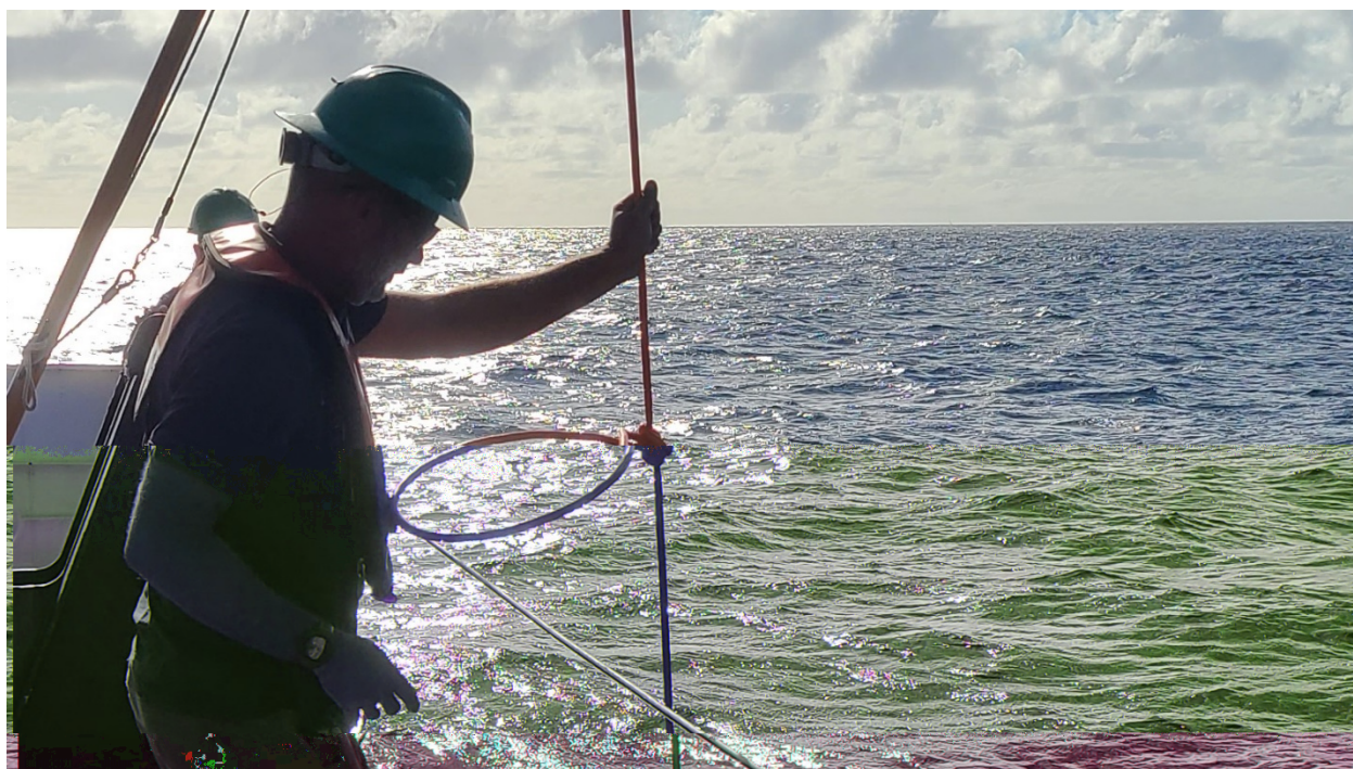
Figure 2. Knot observed on the NILSPIN™ wire immediately below the 500m mark during the 20.5°N, 23°W mooring (PT039) recovery. (Photo: Renellys Perez)
