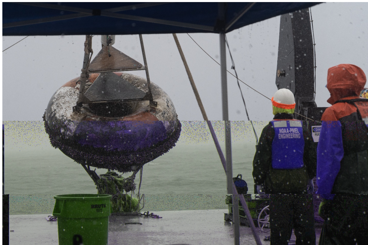
Figure 4. 12°N, 38°W mooring (PI254) recovery. Note rope in bridle (Photo: Grace Owen)
