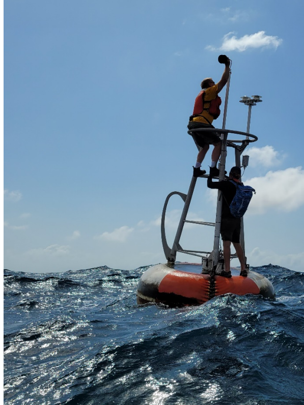
Figure 3. Replacing the wind sensor on 0°, 23°W mooring (PT045b). (Photo: Mark Watson)
