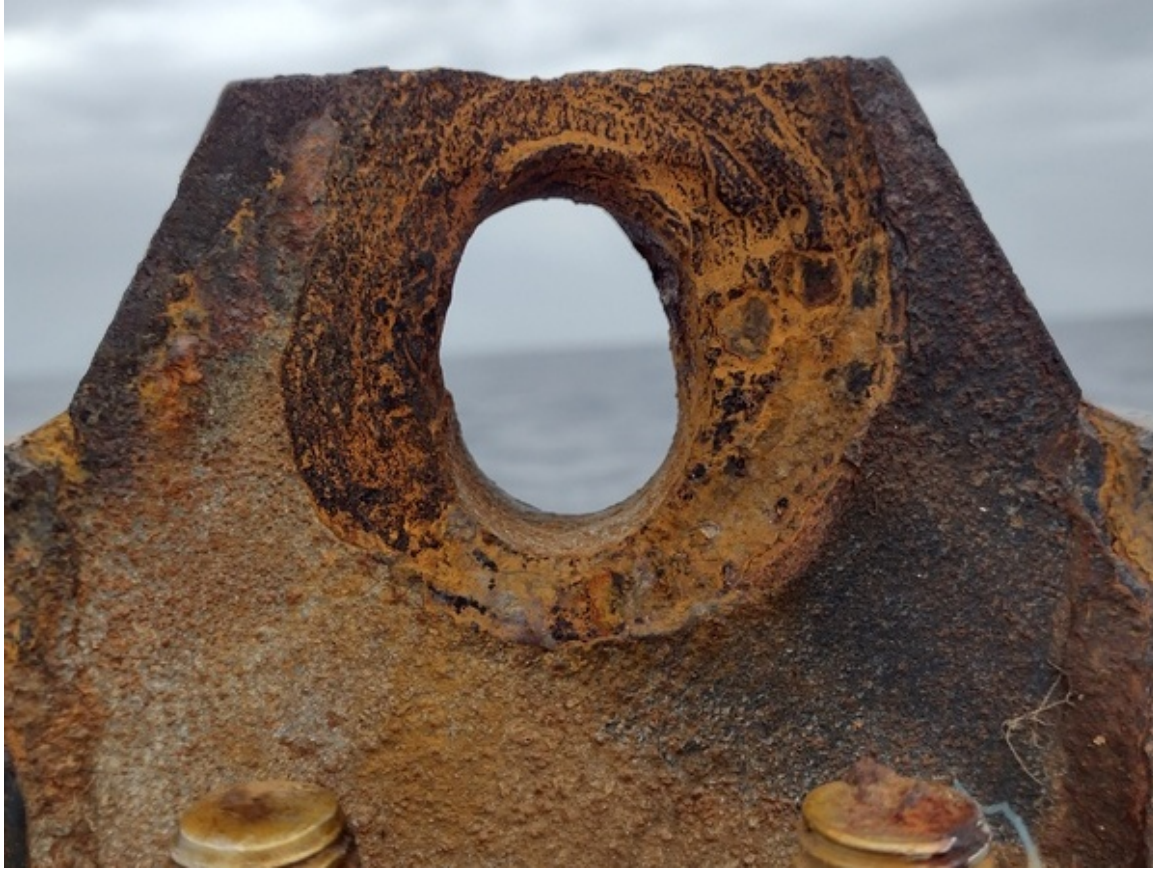
Figure 6. Worn clevis from 12°N, 38°W (PI254) recovery.
