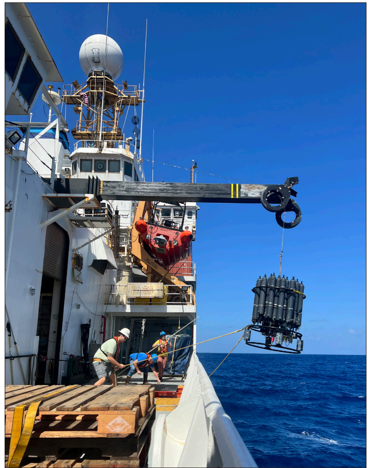
A conductivity-temperature-depth (CTD) instrument is recovered from the Atlantic to be brought aboard the NOAA Ship Ronald H. Brown after a full water column cast. Photo credit: NOAA-AOML.
