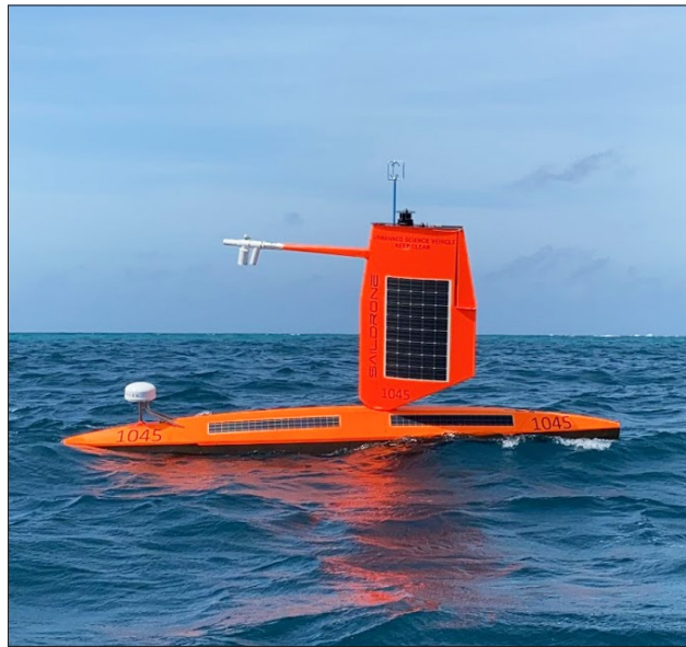
Left: A saildrone surface uncrewed vehicle in the Atlantic. Saildrones are equipped with a special “hurricane wing” to withstand the extreme wind conditions encountered in tropical cyclones as they gather observations from the near-surface ocean and atmosphere in real-time (photo credit: Saildrone). Right: An underwater glider deployed to measure the upper ocean’s properties, with a focus on temperature and salinity, to depths as great as half a mile along predetermined tracks (photo credit: Allan Jones, Cape Eleuthera Island School).
