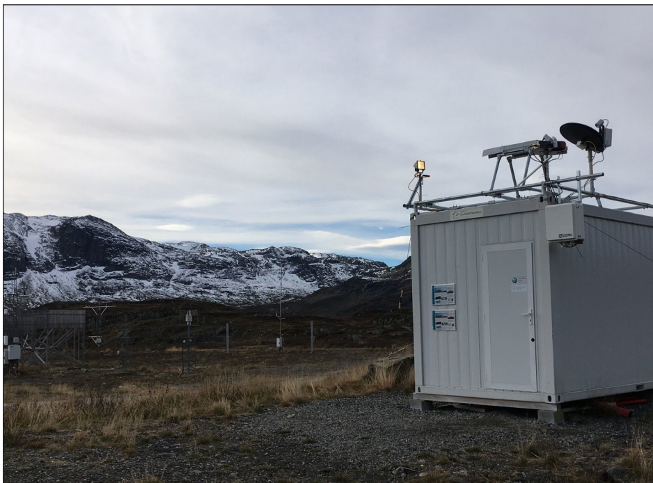
Met Norway snowfall measurement equipment (left, background) and science container (right, foreground). The MRR, PIP, and MASC are mounted on the top of the container. Not a bad spot to spend a snowy winter.
