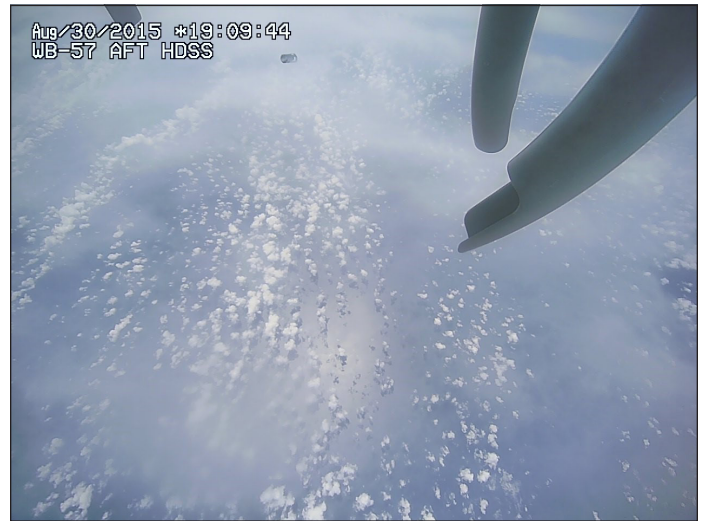
This is a rare photo from rear facing camera of the WB 57, during a mission into Erika, where the camera unbelievably caught the sonde in the air, just after it was released and moving away from the plane.
