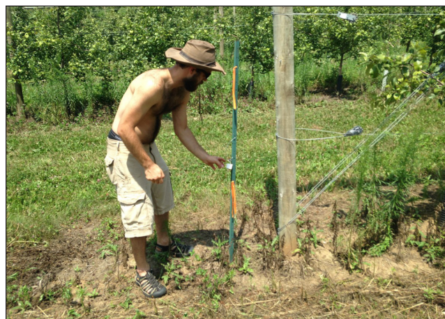
Graduate student Brian Zimmerman works in oppressive heat and humidity (heat index 109!) to check the operation of one of 32 Thermochron sensors deployed around the four Sacia properties. (Photo by Grant Petty)
