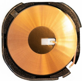
Wireless Charging Coil Gold Copper
