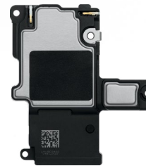
Speaker Steel Copper Rare earth elements
