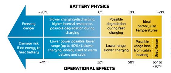
Effects of cold temperatures on batteries and EVs. The top half shows temperature effects on batteries based on physics. The bottom half of the figure shows the operational effects on EV performance. *Source: Cold Weather Impacts on EVs, Michelle Wilber, Alaska Center for Energy and Power*
