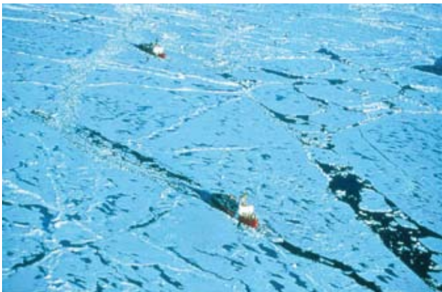
Figure 4.12. Image from a helicopter of icebreakers (125-m length) operating in the central Arctic Ocean through 2-m-thick, multiyear sea ice. Note the linear features (leads), melt ponds on the ice surface, and pressure ridge in the lower left extending to the top of the image. (Photo credit: L.W. Brigham, 1994)
