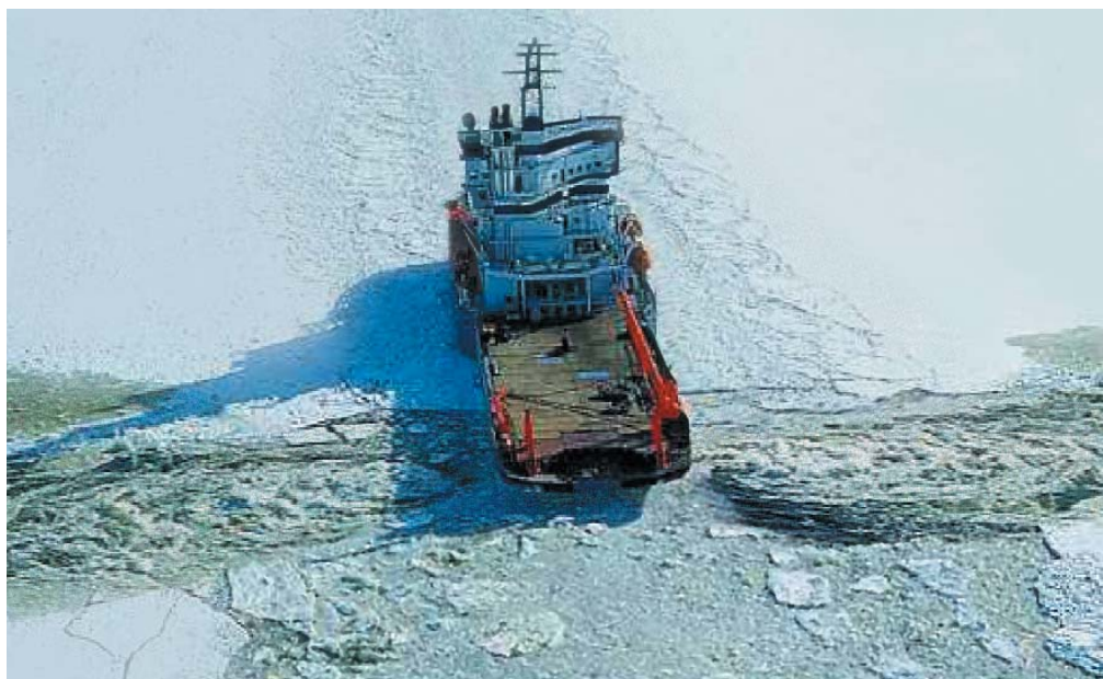
Figure 12 Lateral mixing of ice by the Finnish icebreaker Fennica using azimuthing thrusters to clear a channel. Photo: Aker Finnyards
