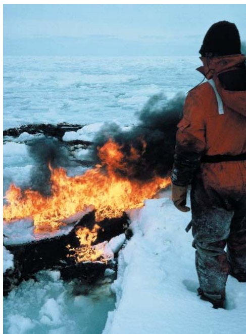
Figure 9 Burning crude oil in slush-filled lead off Nova Scotia, Canada, 1986. Photo: SL Ross and DF Dickens, 1987
