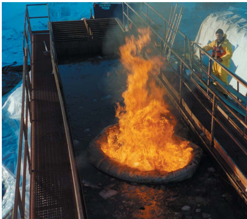
Figure 3 Burning in brash ice, ACS wave tank at Prudhoe Bay, Alaska, October 2002 (Buist et al., 2003)
