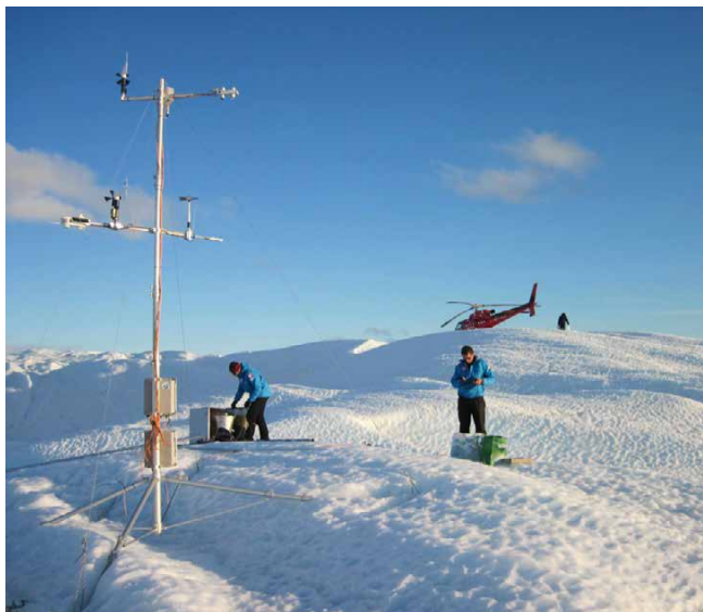
Installing an Automatic Weather Station in Greenland. Photo: Paul Smeets
