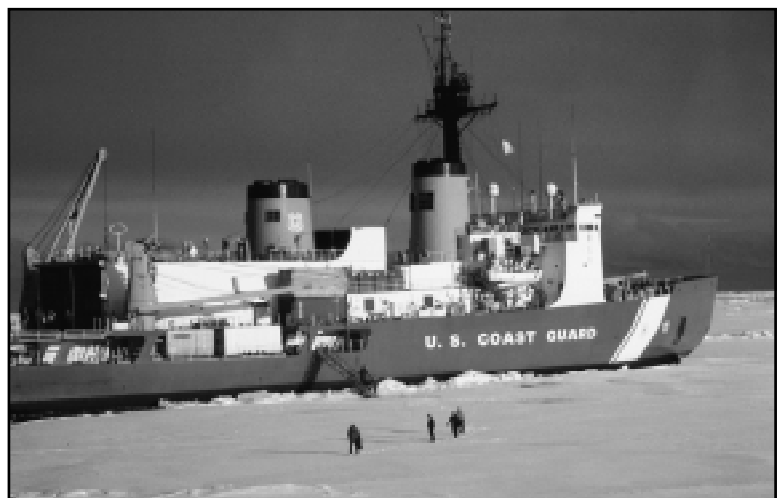
The USCG Polar Sea during the 1994 Arctic Ocean Section cruise. The U.S. Coast Guard's two 399-foot Polar Class icebreakers have supported a number of oceanography, geology, geophysics, sea-ice, and biology studies (photograph by Lawson Brigham).
