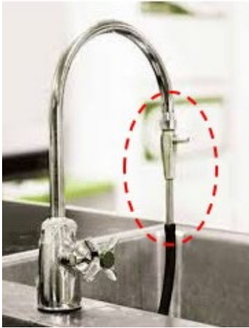
Figure 8.7. Water-driven aspirator vacuum pump - historically used in high-school chemistry classes.
