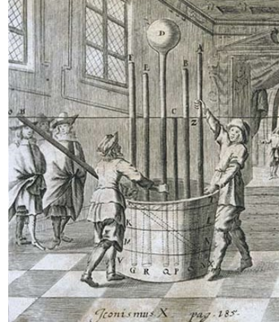
Figure 8.1. c. 1700’s image of Torricellian Columns indicating identical Hg column heights independent of tube length. Note evacuated bulb on central column.
