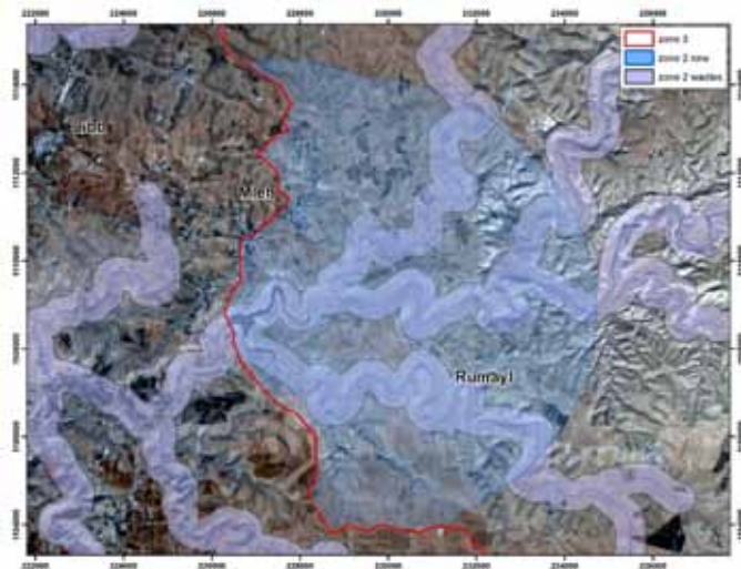
Figure 4: Surface Water Protection Zones for the Wadi Wala Dam (according to the Jordanian guideline zone 2 for main wadis covers a buffer zone of 350 m to both sides of the center of the wadi)
