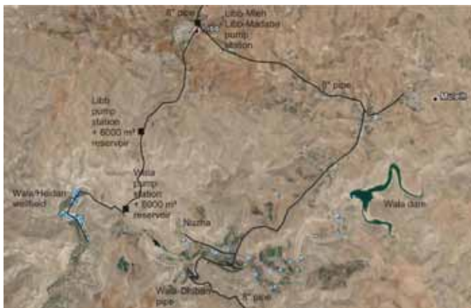
Figure 5: Locations of Wadi Wala Dam and Wala/Heidan Well Field with Water Supply Network (the green areas between the reservoir and the well field indicate irrigated areas)
