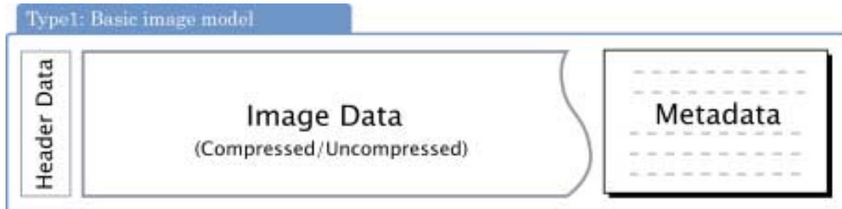
Figure 2-2: Basic conceptual structure of a digital image
