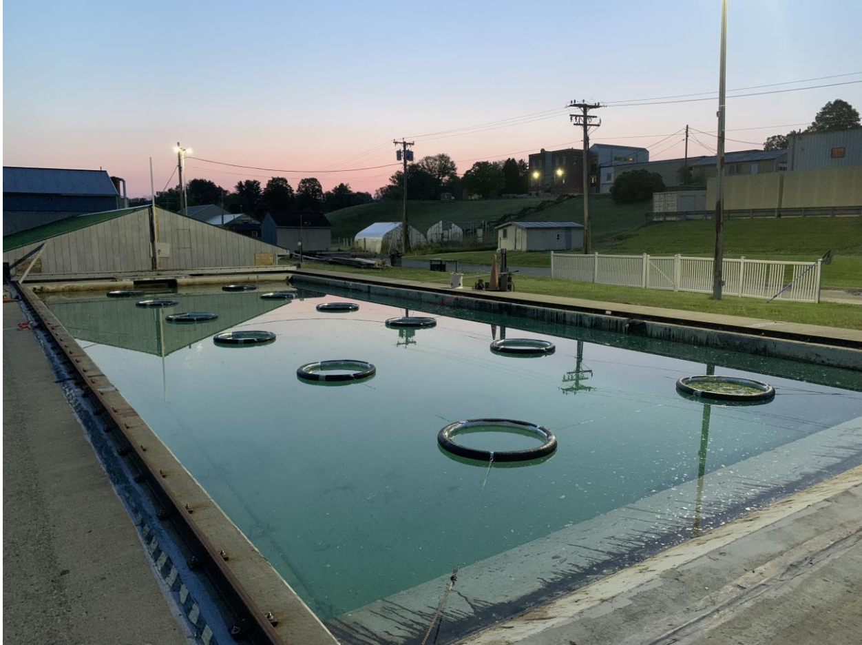
Fig. 24 CRREL test pool at sunset showing oil targets and cover
