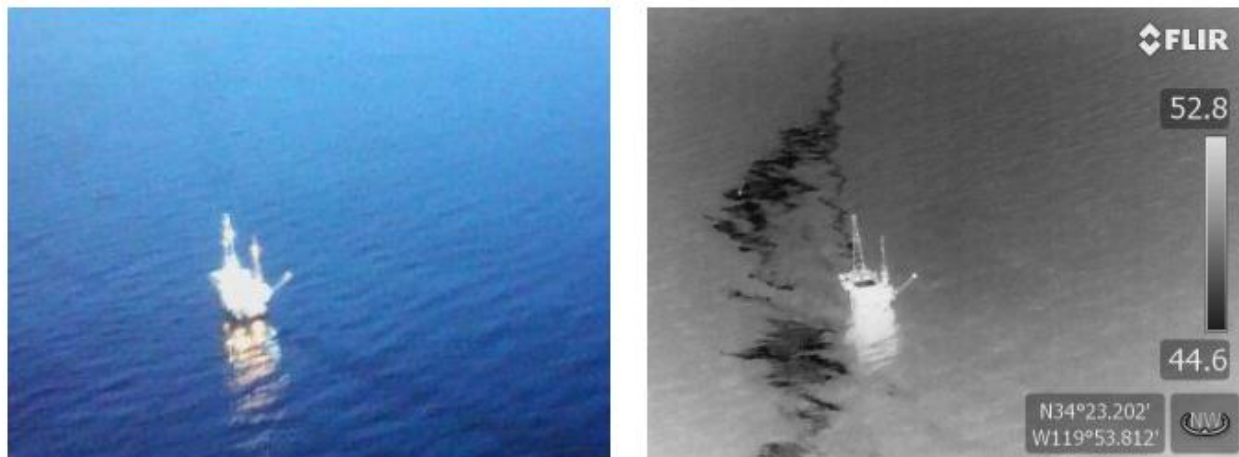
Fig. 4 Imagery from FLIR Systems T650sc LWIR camera (right) showed significant oil compared to visible imagery (left)
