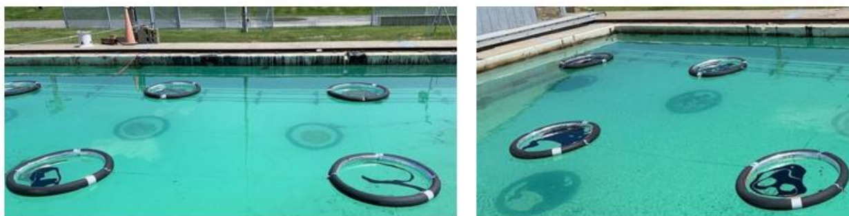
Fig. 27 CRREL test pool with oil targets
