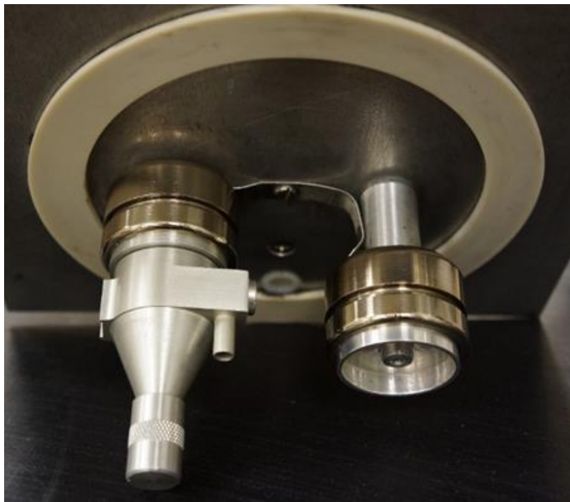
Figure 6. Metallic aerosol samplers attached to the underside of the UNC Venturi containment chamber lid (photo provided by D.E. Evans, NIOSH). The respirable GK2.69 cyclone sampler is on the left and the total dust closed-face Slaton cassette is on the right. Both samplers are in contact with the center grounding clip.
