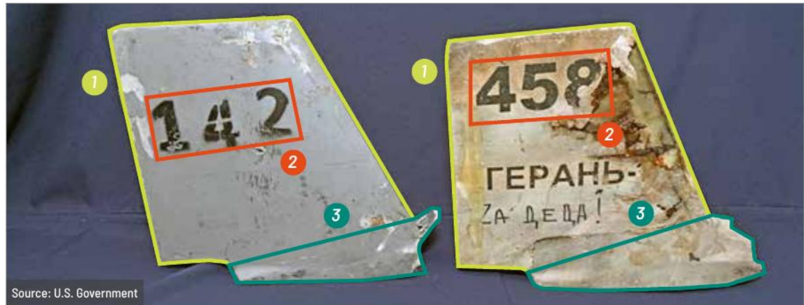
Left: A Shahed-131 wing stabilizer recovered from an attack in Iraq that Iran claimed, September 2022 Right: A Geran-1 wing stabilizer recovered in Ukraine, fall 2022
