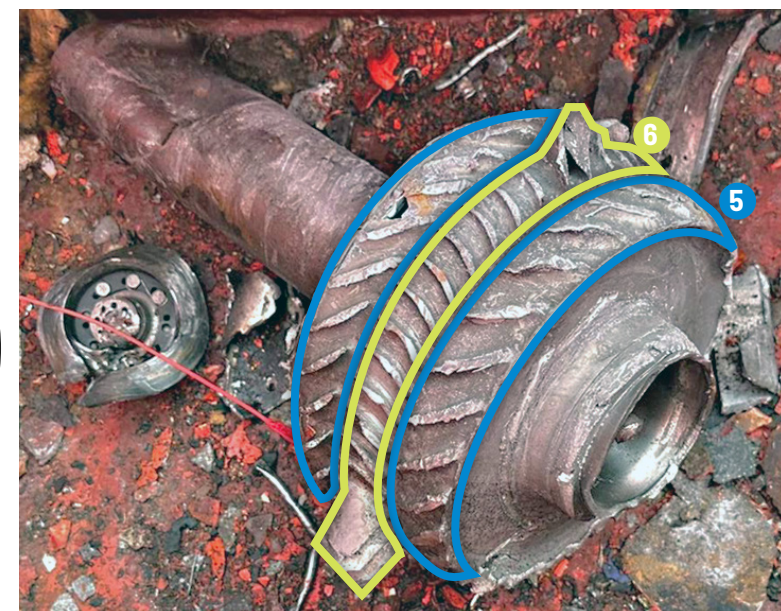
The turbojet engine debris recovered from the M/V Strinda are consistent with the Iranian Tolu-4 from the Noor ASCM
