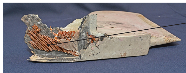
Underside of the Shahed-131 (Geran-1) recovered in Ukraine showing distinctive honeycomb design
