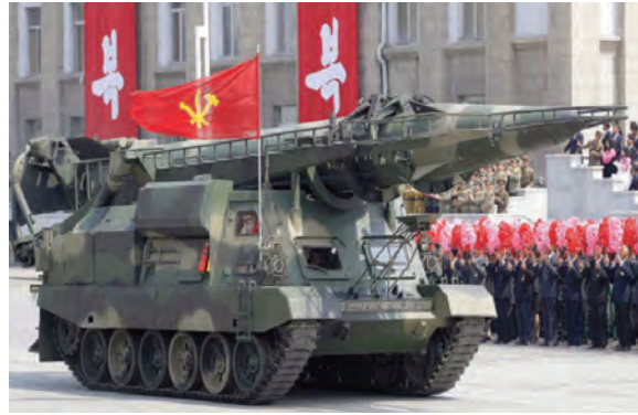
Scud class SRBM on new tracked launcher, paraded in Pyongyang in April 2017.
