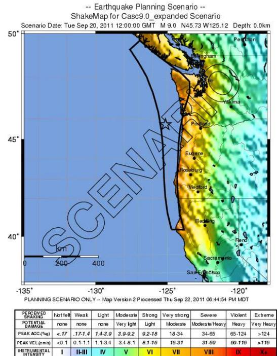
Figure 1. ShakeMap for a M9.0 earthquake on the Cascadia megathrust. The black polygon offshore is the modeled fault rupture for this scenario.
