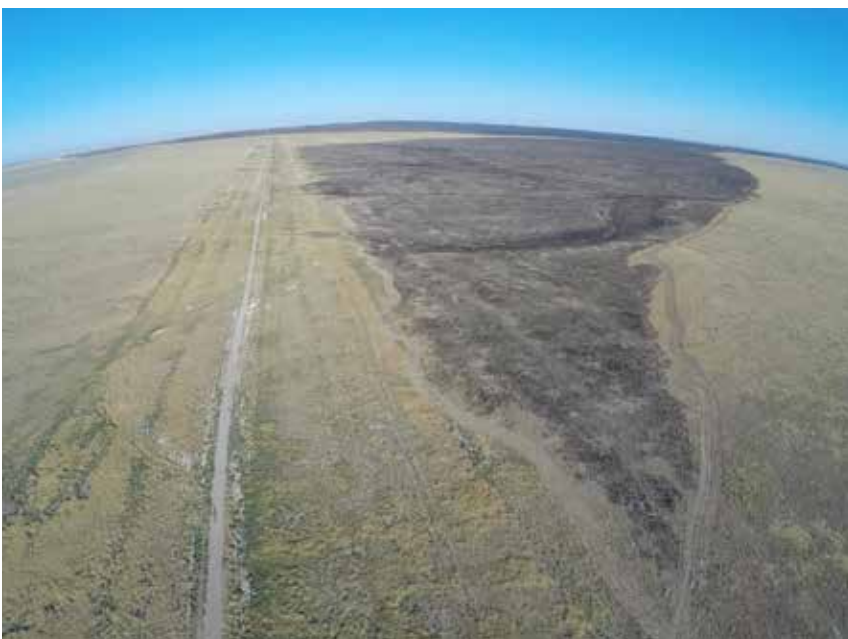
Fuel breaks along a road in southern Idaho slowed the progression of the Pot Hole Fire long enough so that firefighters could build a containment line around it.
