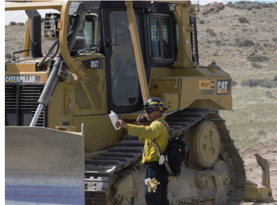
Primed for action: students from the BLM's Dozer Academy practice creating dozer lines while constructing 30 miles of fuels breaks at Utah's Dugway Proving Grounds. Dozer lines remove brush and debris that might fuel the spread of fire. (BLM/Mike Hislop)
