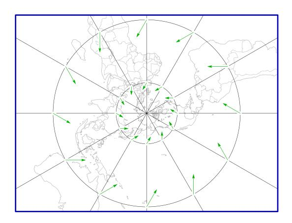
➤ Example 7: Another plotting example, this time with the Orthographic Projection. We chose a point on the Earth with latitude 40° and longitude 105°. This point will be in the center of the map. We then took **A** to be the east vector **E** for that location, and then **B** to be the north vector **N** there. As in the previous example, we took the vector field to have a constant bearing of 30° and a constant magnitude.
