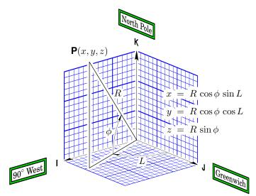
From the figure above, we have  $\mathbf{P}=R\begin{bmatrix}\cos\phi\sin L\\\cos\phi\cos L\\\sin\phi\end{bmatrix}$ . Differentiating this with respect to  $\phi$  gives  $\begin{bmatrix}-\sin\phi\sin L\end{bmatrix}$
