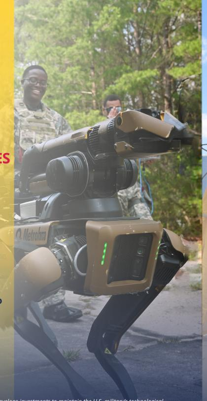
(Background) DTRA delivers science, technology and capability that develops investments to maintain the U.S. military's technological superiority in countering WMD. The robotic dog, seen here, is retrofitted with chem-bio sensors that allows joint forces to safely assess threat levels in unknown areas.
