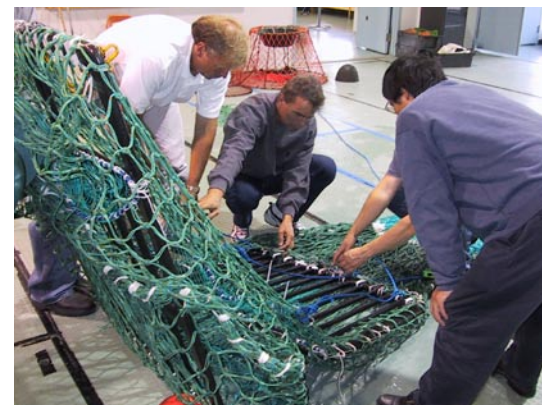
Pingguo He, right, back to camera, works with fishermen from Poland, Maine, on a fishing net designed to catch flat fish, but let cod escape.
