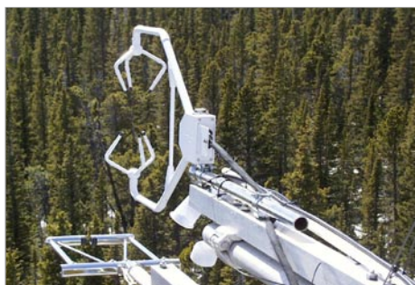
The Colorado University AmeriFlux tower near Niwot Ridge, Colorado. At top is a sonic anemometer, which measures fluctuations of vertical and horizontal wind. The krypton hygrometer below measures rapid fluctuations in water vapor. Photo courtesy of Sean Burns.
