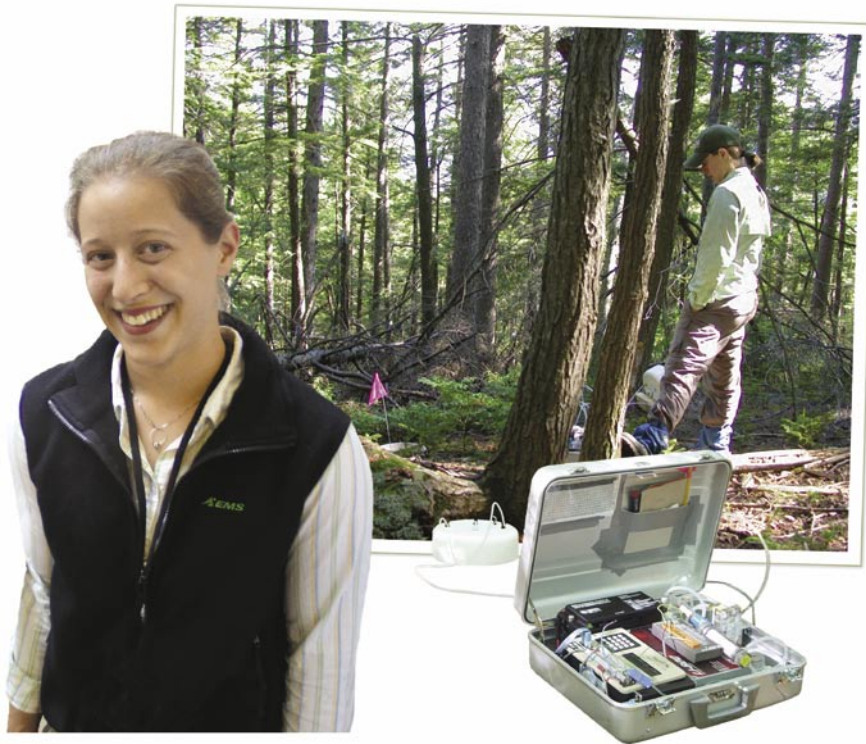
Sarah Silverberg uses a portable infrared gas analyzer to measure soil carbon levels at the Bartlett Experimental Forest.
