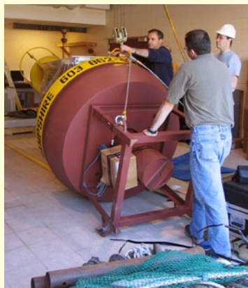
A state-of-the-art coastal ocean observing buoy being assembled in an EOS high-bay area prior to deployment in Great Bay.
