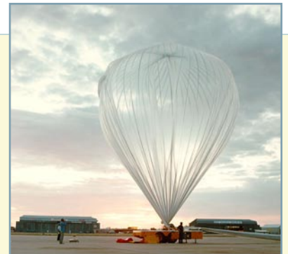
A balloon like this, thinner than a garbage bag and filled with six million cubic feet of helium, will haul the 2.5 ton BalloonWinds payload aloft to 100,000 ft.
