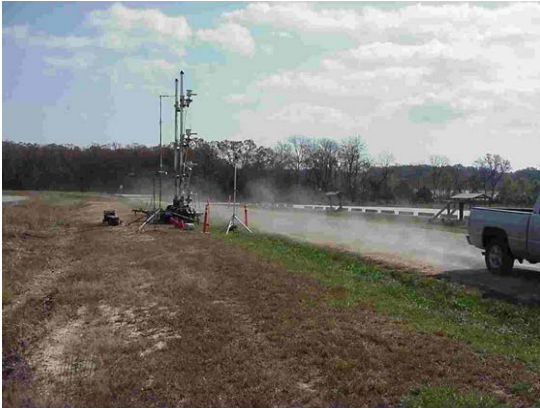
Figure 7. Deployment of Collocated Plume Profiling Towers at Roadside Location
