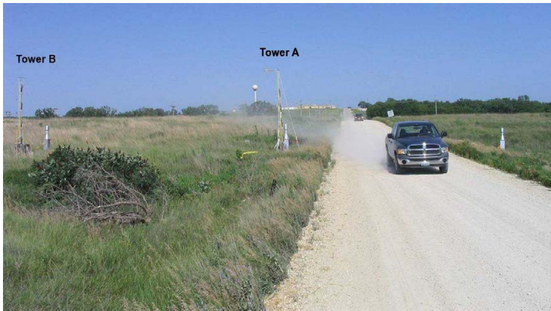
Figure 8A. Example deployment of plume profiling towers at distances of 5 m (Tower A) and 25 m (Tower B) from an unpaved road in tall grass area [7]
