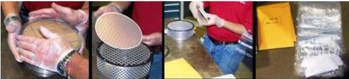
Figure 12. Removing Fume Sample from Weld Fume Chamber
