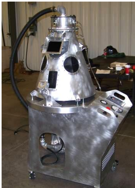
Figure 1. NSRP Weld Fume Chamber
