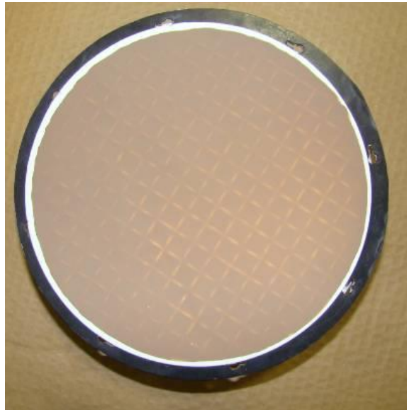
Figure 10. Filter That Would Pass Inspection Demonstrating No Fume Was Lost
