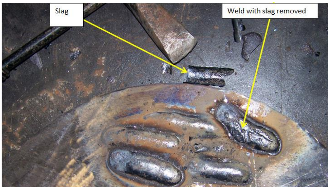
Figure 1. Slag chipped off of welds on test plate.
