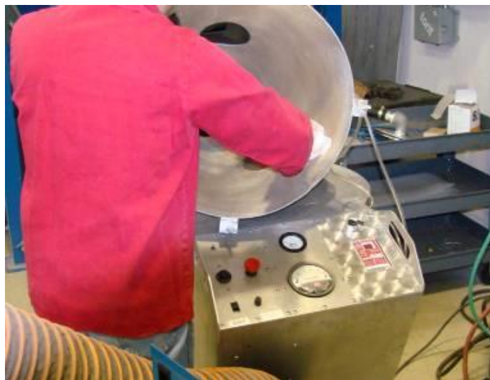
Figure 14. Cleaning the Chamber between runs
