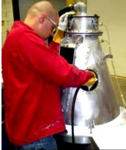
Figure 8. Welding Inside Weld Fume Chamber
