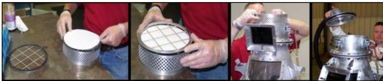
Figure 7. Placing Filter in Weld Fume Chamber
